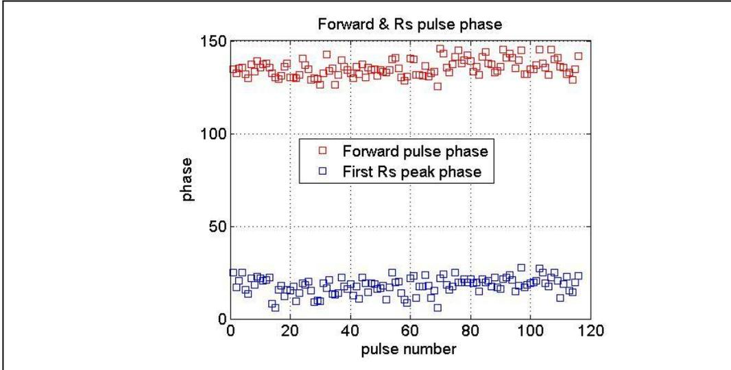
Figure 8: The forward RF phase(red) and the reflected RF phase at the first peak(blue) for normal pulse during the T24\_disk\_#3 RUN2.
