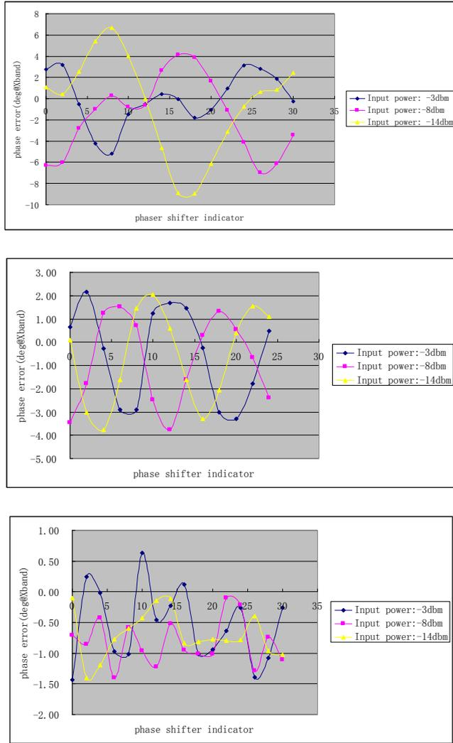
Figure 4: the deviations of the output phase to the input phase. From top to bottom: without calibration; With incomplete calibration (only DC offset is subtracted); fully calibration.
