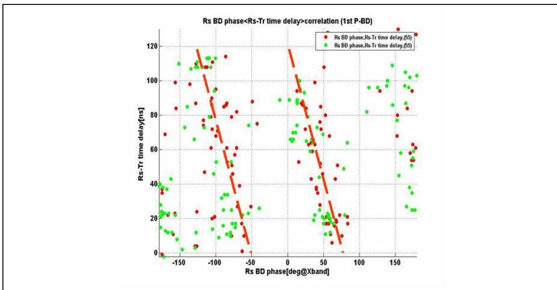
Figure 10: The breakdown phase distribution as a function of the Rs-Tr time delay. The red is ACC-breakdown type, and the green is the 1<sup>st</sup> pulse breakdown. The forward RF pulse width is 252ns.
