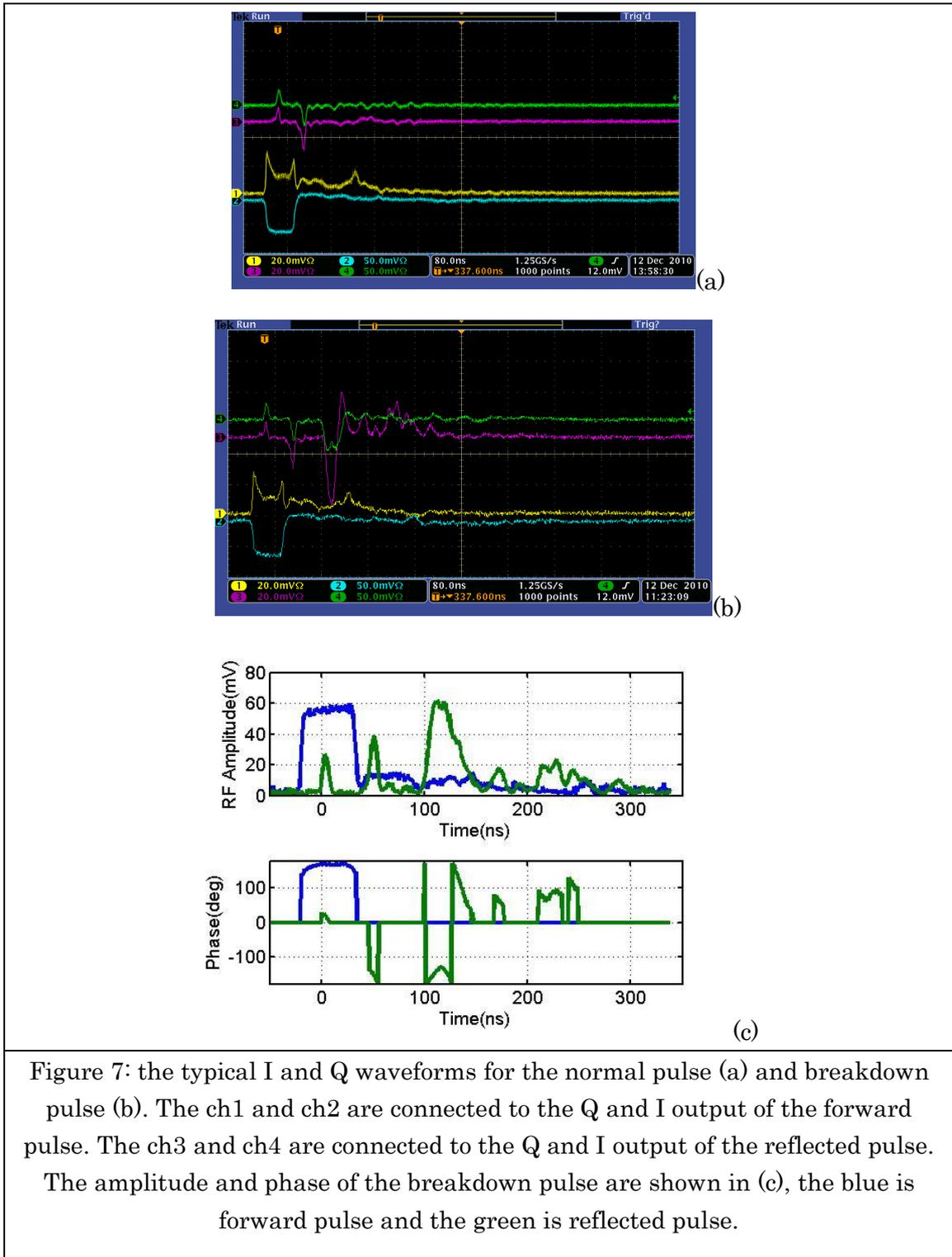
Figure 7: the typical I and Q waveforms for the normal pulse (a) and breakdown pulse (b). The ch1 and ch2 are connected to the Q and I output of the forward pulse. The ch3 and ch4 are connected to the Q and I output of the reflected pulse. The amplitude and phase of the breakdown pulse are shown in (c), the blue is forward pulse and the green is reflected pulse.
