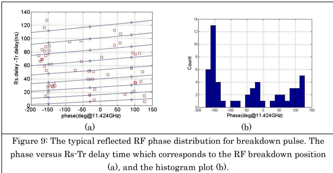
Figure 9: The typical reflected RF phase distribution for breakdown pulse. The phase versus Rs-Tr delay time which corresponds to the RF breakdown position (a), and the histogram plot (b).
