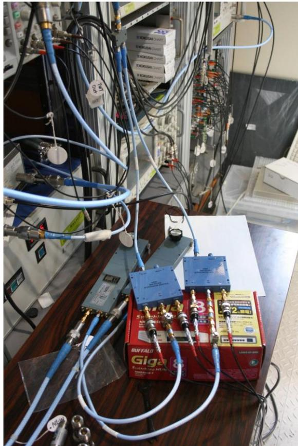
Figure 6: preliminary setup for T24 reflected RF phase measurement.
